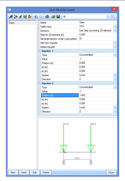
With **Sections**, the option **Use step according 2D element** is chosen with **0,25m** as step. To have both rails of the train track, a second impulse is added trough the option **Add new impulse**. The position of the second impulse is **1,4m**.
