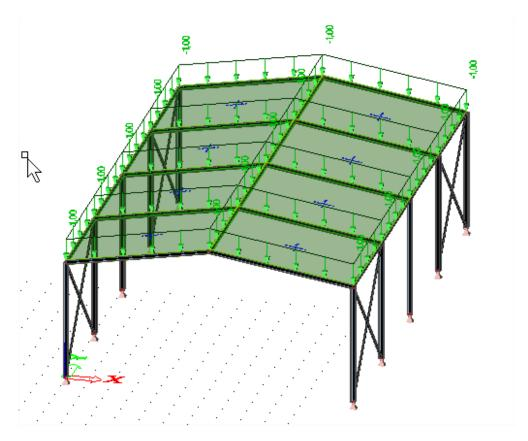
These area loads need to be distributed to the nodes of the load panels. This can be done by selecting the load panels and using the action **Generate loads**.
