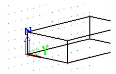
It is the intention to load all walls (4 walls of the rectangular pool and 1 wall of the circular pool), by only introducing one free surface load. To be able to do this, the Z axis of the LCS of all walls, needs to be pointing to the inside of the pool. In this project, this is already done by changing the LCS of 2 walls by inserting the surface supports.
