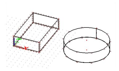
Surface supports are always placed on the negative site of the local Z axis of the 2D element. For that reason, the positive direction of the local Z axis for each wall element should be pointing towards the inside of the pool. If this is not the case, the option **Swap Orientation** can be used in the property window of the 2D element.
