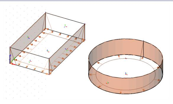
Now all walls are loaded by the water pressure, by inserting only one free surface load.
