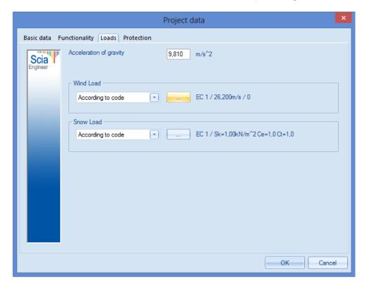
There are three types of climatic load generators for 2D frames in Scia Engineer:
