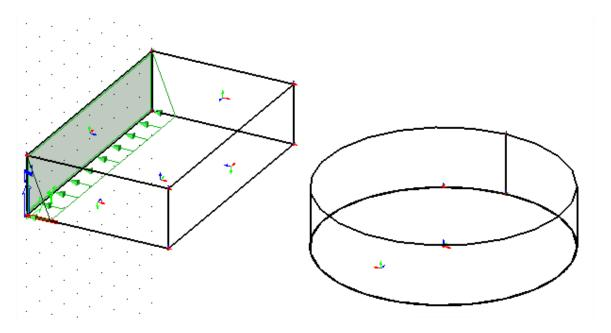
Since all walls need to be loaded by this water pressure, the walls can be selected using the action **Update 2D member selection** in the property window of the free surface load. To end the selection functionality, click **Esc**.
