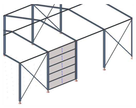
This load panel will be loaded with a surface load of  $-0.30 \text{ kN/m}^2$  in the global X direction (load case – X):
