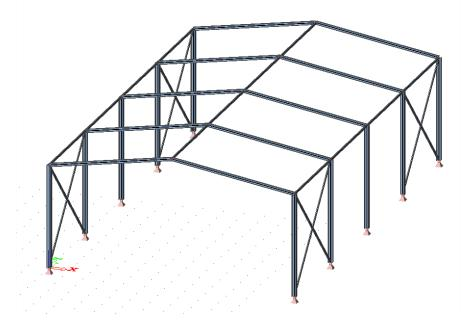
The self weight of the structure is automatically calculated by Scia Engineer. The weight of the roof will be inserted manually using the **Plane generator** in the Load menu.
