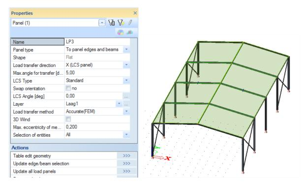
These load panels will be loaded with an area load of -1 kWm². The loads can be inserted in the Load menu with the option Surface load, on 2D member.
