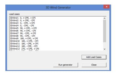
Afterwards, the generating of the loads in these load cases can be started by using the option **Run generator.**
