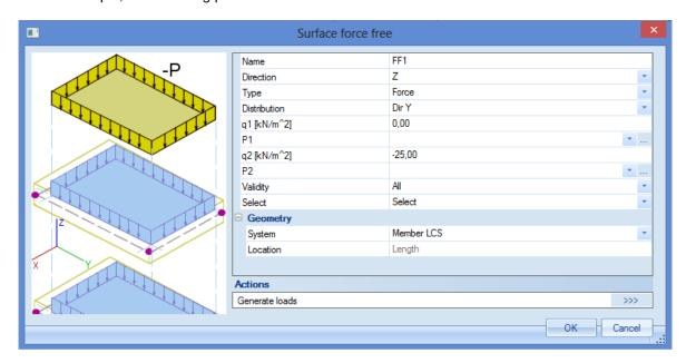
Since the value of the loads has to be 0 at the top and -25 at the bottom, it is necessary to use this order of nodes by drawing the free surface load:
