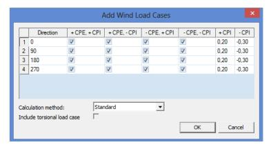
By default, **16 load cases** are generated. Four cases for each wind direction. For the **Load Coefficients**, the Cpe values are taken from the code (EN 1991-1-4, see Chapter 2D Wind generator [1]), the Cpi coefficients needs to be inserted manually.
