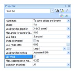
This means that **Wind data** will be created on the load panels. This wind data is shown as a small blue arrow. By selecting this arrow, the properties can be viewed and changed.
