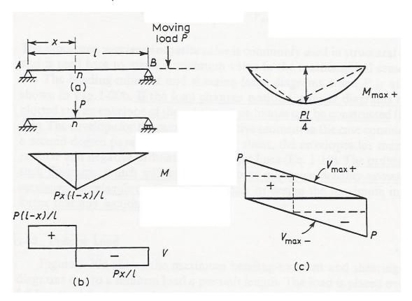
Figure (a) represents a simple beam on 2 supports, across which a concentrated load P can move.
