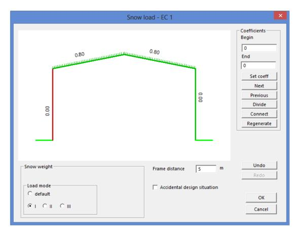
After clicking on OK in this window, the snow load 1 will be generated on the roof elements. The same can be done for Snow load 2 and 3.
