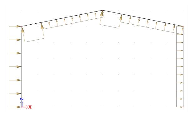
The Load Coefficients are calculated according to the code, EN 1991-1-4.
