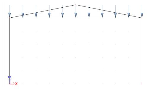
The **Load Coefficients** are calculated according to the code, EN 1991-1-3. Table 5.2 [2] is used for the load coefficients.
