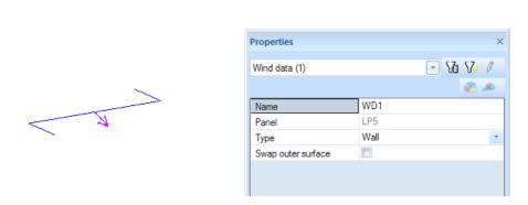
It is necessary that the arrows are pointing in the direction outside the structure. For that reason, there are two Wind Data for which the option **Swap outer surface** has to be marked.
