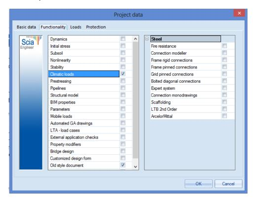
In the next tab, the wind and snow load should be chosen (according to the code or user defined).
