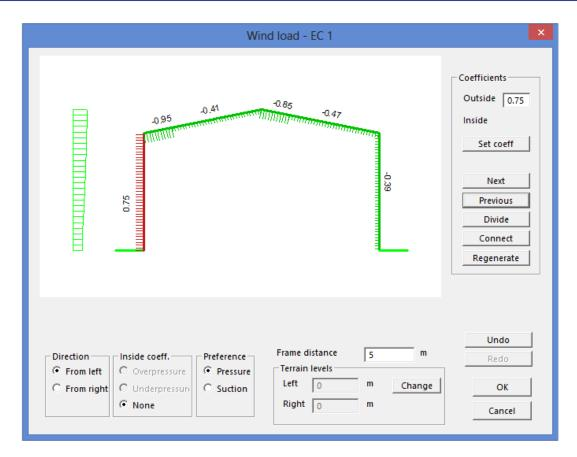
For the load case Wind Left, the direction is set to 'From left'.
