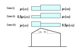
Figure 5.3: Snow load shape coefficients - pitched roofs
