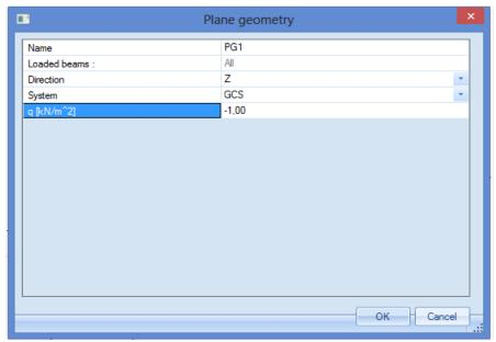
By inserting an area load using the plane generator, all beams in the specified plane are loaded. This can be changed afterwards.
