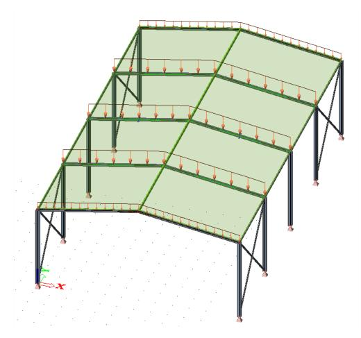
Since the **Accurate (FEM)** load transfer method is used, the loads are generated correctly without the need for the user to insert the load factors.
