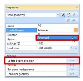
With the option **Update beams selection**, all beams that have to be loaded can be selected.
