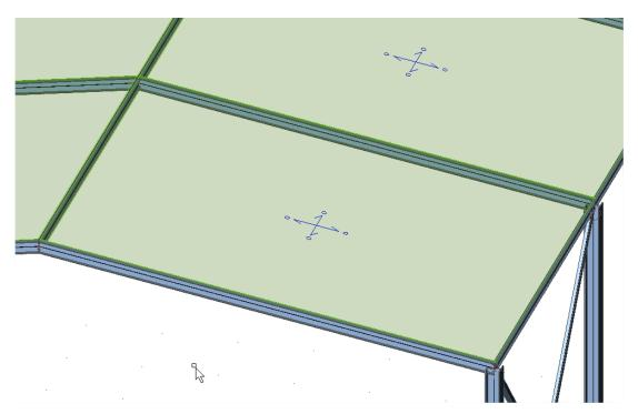
An area load of -1  $kN/m^2$  will be placed on each load panel. This can be done in the Load menu, using the option **Surface load, on 2D member**.
