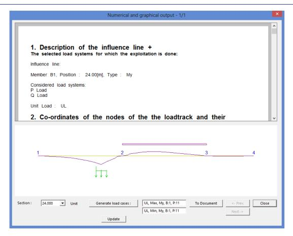
Through the button **Generate Load Cases** two load cases are generated, one for the minimal My on 24m and one for the maximal My on 24m. The parameter B indicates the member, parameter P the position on the member.
