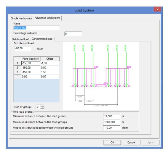
The load system consists of 2 groups of three point loads and a divided load. The point loads have a value of 150 kN and a mutual distance 1.5m. The divided load has a value of 80 kN/m.
