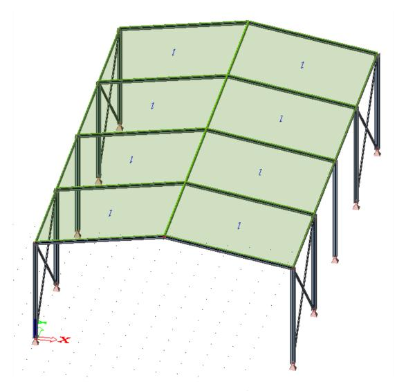
These load panels will be loaded with area loads of -1  $kN/m^2$ . This can be done in the Load menu using the option Surface load, on 2D member.
