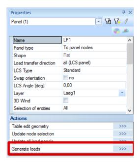
Afterwards, the point forces are generated on the nodes of the load panels.
