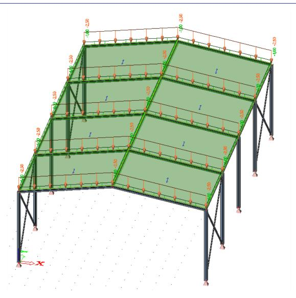
Since the beams in the middle of the roof have a load panel on each side, these beams are loaded twice with the same line load.
