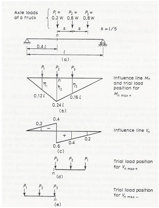
Figure (a) represents a simple beam on two supports again. Across the beam, a system of three point loads can move which represent e.g. the axis loads of a lorry. We look for the position of the load system for which the moment and the shear force are maximal in the section "n".
